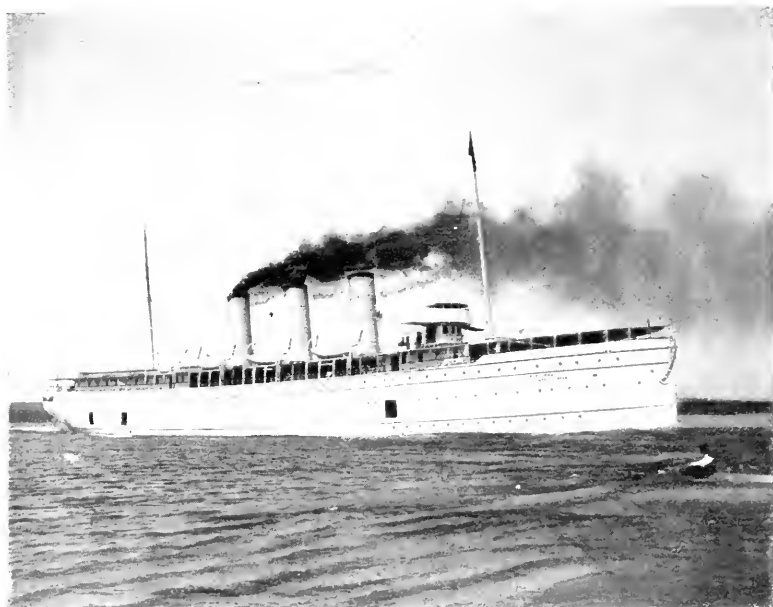
STR. NORTH LAND, 4244 TONS, NORTHERN S. S. CO. Length 353 feet, breadth 41, depth 26. Built by Globe Iron Works, Cleveland, O.
